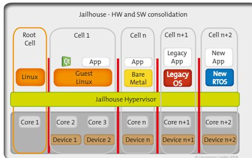
Fig. 2: System consolidation with jailhouse
